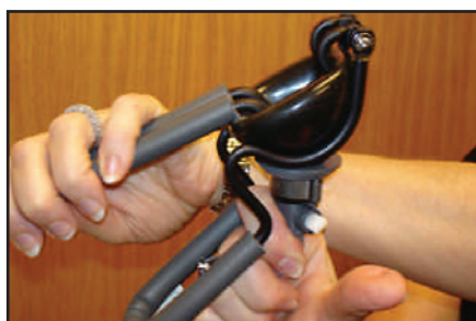
Release purge valve.
