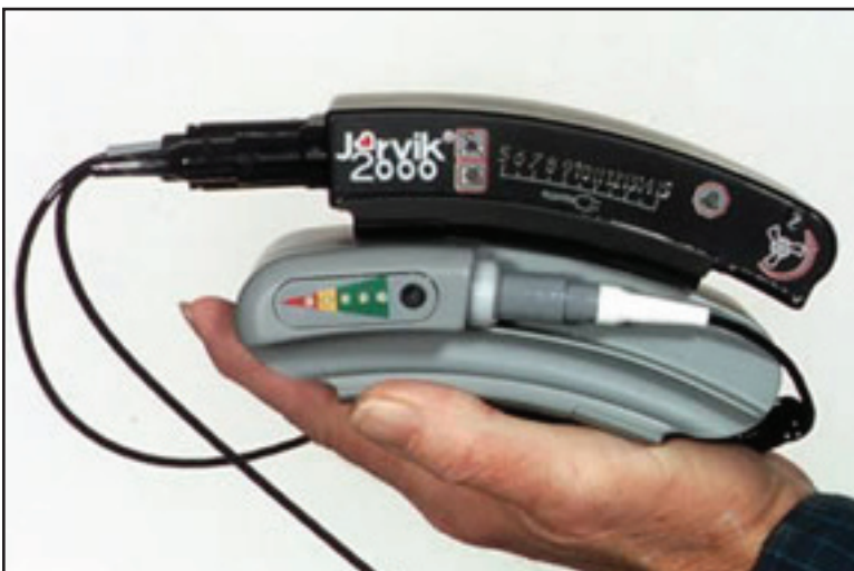
Controller attached to the portable Li-ion battery.
